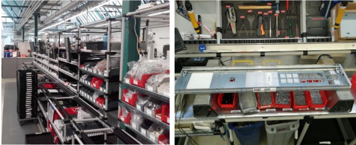
Figure 8: Current set-up with separate kitting, assembly and testing workstations
