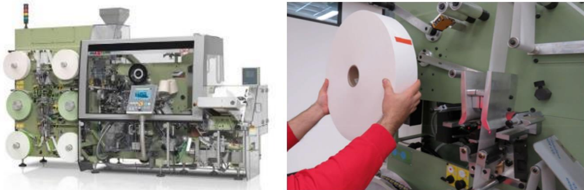
Figure 5: C24-E tea bag packaging machine - lifting a reel to the upper position.
