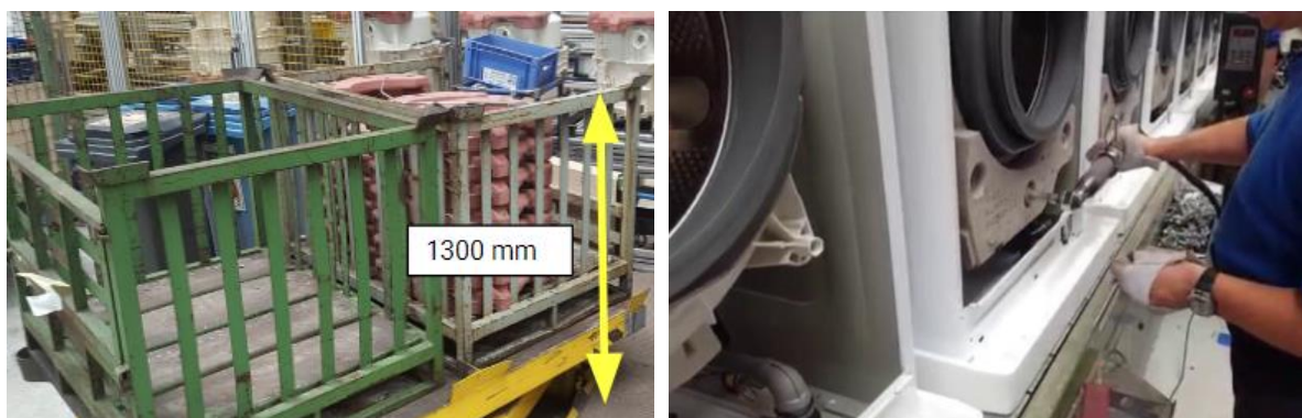
Figure 3: Left - the bins from which the counterweights are picked up; right - fixating a counterweight to the washing machine
